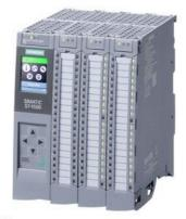
SIMATIC S7-1500 Compact CPU CPU 1512C-1 PN, central processing unit with working memory 250 KB for program and 1 MB for data, 32 digital inputs, 32 digital outputs, 5 analog inputs, 2 analog outputs, 6 high speed counters, 4 high speed outputs for PTO/PWM/frequency output 1. interface: PROFINET IRT with 2 port switch, 48 NS bit-performance, incl. front connector push-in, SIMATIC memory card necessary
