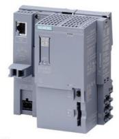
SIMATIC DP, CPU 1510SP F-1 PN for ET 200SP, central processing unit with 300 KB work memory for program and 1 MB for data, 1st interface: PROFINET IRT with 3-port switch, 25 ns bit performance, SIMATIC Memory Card required, BusAdapter required for port 1 and 2
