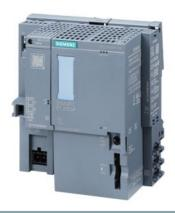
SIMATIC DP, CPU 1510SP-1 PN for ET 200SP, central processing unit with work memory 200 KB for program and 1 MB for data, 1st interface: PROFINET IRT with 3-port switch, 25 ns bit performance, SIMATIC Memory Card required, BusAdapter required for port 1 and 2
