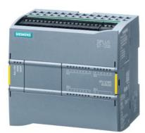
SIMATIC S7-1200F, CPU 1214 FC, compact CPU, DC/DC/relay, onboard I/O: 14 DI 24 V DC; 10 DO relay 2 A; 2 Al 0-10 V DC, power supply: DC 20.4-28.8 V DC, program/data memory 200 KB
