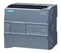
SIMATIC S7-1200, CPU 1214C, compact CPU, DC/DC/DC, onboard I/O: 14 DI 24 V DC; 10 DO 24 V DC; 2 AI 0-10 V DC, power supply: DC 20.4-28.8 V DC, program/data memory 150 KB
