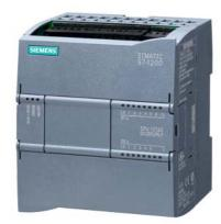
SIMATIC S7-1200, CPU 1212C, compact CPU, DC/DC/relay, onboard I/O: 8 DI 24 V DC; 6 DO relay 2 A; 2 AI 0-10 V DC, power supply: DC 20.4-28.8 V DC, program/data memory 100 KB
