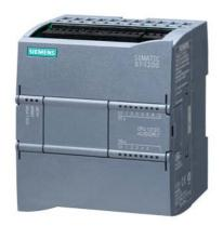
SIMATIC S7-1200, CPU 1212C, compact CPU, AC/DC/relay, onboard I/O: 8 DI 24 V DC; 6 DO relay 2 A; 2 AI 0-10 V DC, power supply: AC 85-264 V AC at 47-63 Hz, program/data memory 100 KB
