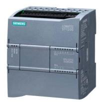
SIMATIC S7-1200, CPU 1211C, compact CPU, DC/DC/DC, onboard I/O: 6 DI 24 V DC; 4 DO 24 V DC; 2 AI 0-10 V DC, power supply: DC 20.4-28.8 V DC, program/data memory 75 KB
