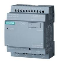
LOGO! 12/24RCEO, logic module, PS/I/O: 12/24VDC/relay, 8 DI (4 AI)/4 DQ, without display, memory 400 blocks, modular expandable, Ethernet, integrated web server, data log, user-defined web pages, standard microSD card for LOGO! Soft Comfort V8.3 or higher, older projects executable cloud connection in all LOGO! 8.3 hasic units
