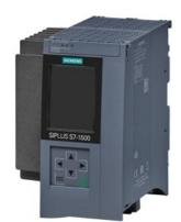
SIPLUS S7-1500 CPU 1516F-3 PN/DP rail based on 6ES7516-3FN02-0AB0 with conformal coating, -40...+70 °C, OT4 with ST1/2 (+85 °C for 10 minutes), heat sink, no PS usable, central processing unit with work memory 1.5 MB for program and 5 MB for data, 1st interface: PROFINET IRT with 2-port switch, 2nd interface: PROFINET RT, 3rd interface: PROFIBUS, 10 ns bit performance, SIMATIC Memory Card required
