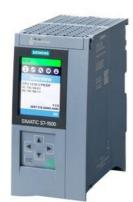
SIPLUS S7-1500 CPU 1516-3 PN/DP rail based on 6ES7516-3AN02-0AB0 with conformal coating, -40...+70 °C, OT4 with ST1/2 (+85 °C for 10 minutes), heat sink, no PS usable, central processing unit with work memory 1 MB for program and 5 MB for data, 1st interface: PROFINET IRT with 2-port switch, 2nd interface: PROFINET RT, 3rd interface: PROFIBUS, 10 ns bit performance, SIMATIC Memory Card required
