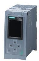
SIPLUS S7-1500 CPU 1515R-2 PN TX rail based on 6ES7515-2RM00-0AB0 with conformal coating, -40...+70 °C, OT4 with ST1/2 (+85 °C for 10 minutes), heat sink, no PS usable, central processing unit without display with work memory 500 KB for program and 3 MB for data, 1st interface: PROFINET with 2-port switch, 2nd interface: PROFINET RT, SIMATIC Memory Card required
