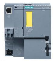
SIPLUS ET 200SP CPU 1512SP F-1 PN T1 rail based on 6ES7512-1SK01-0AB0 with conformal coating, -25...+60 °C, OT1 with ST1/2 (+70 °C für 10 minutes), central processing unit with work memory 300 KB for program and 1 MB for data, 1st interface, PROFINET IRT with 3-port switch, 48 ns bit performance, SIMATIC Memory Card required, BusAdapter required for port 1 and 2
