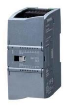
SIPLUS S7-1200 SM 1222 8DQ T1 rail based on 6ES7222-1BF32-0XB0 with conformal coating, -25...+70 °C, OT1 with ST1/2 (+70 °C für 10 minutes), digital output 8 DQ, 24 V DC, transistor 0.5 A
