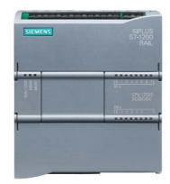
SIPLUS S7-1200 CPU 1212C DC/DC/DC T1 rail based on 6ES7212-1AE40-0XB0 with conformal coating, -25...+60 °C, OT1 with ST1/2 (+70 °C für 10 minutes), compact CPU, DC/DC/DC, onboard I/O: 8 DI 24 V DC 6 DQ 24 V DC 2 AI 0-10 V DC, power supply: 20.4-28.8 V DC program/data memory 50 KB
