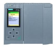
SIPLUS S7-1500 CPU 1518F-4 PN/DP based on 6ES7518-4FP00-0AB0 with conformal coating, 0...+60 °C, central processing unit with work memory 4.5 MB for program and 10 MB for data, 1st interface: PROFINET IRT with 2-port switch, 2nd interface, Ethernet, 3rd interface, Ethernet, 4th interface, PROFIBUS, 1 ns bit performance, SIMATIC Memory Card required
