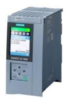
SIPLUS S7-1500 CPU 1516F-3 PN/DP based on 6ES7516-3FN02-0AB0 with conformal coating, -40...+60 °C, central processing unit with work memory 1.5 MB for program and 5 MB for data, 1st interface: PROFINET IRT with 2-port switch, 2nd interface: PROFINET RT, 3rd interface: PROFIBUS, 10 ns bit performance, SIMATIC Memory Card required
