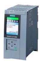
SIPLUS S7-1500 CPU 1516-3 PN/DP based on 6ES7516-3AN02-0AB0 with conformal coating, -40...+60 °C, central processing unit with work memory 1 MB for program and 5 MB for data, 1st interface: PROFINET IRT with 2-port switch, 2nd interface: PROFINET RT, 3rd interface: PROFIBUS, 10 ns bit performance, SIMATIC Memory Card required
