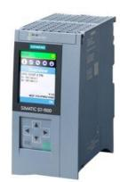
SIPLUS S7-1500 CPU 1515F-2 PN based on 6ES7515-2FM02-0AB0 with conformal coating, -40...+60 °C, central processing unit with work memory 750 KB for program and 3 MB for data, 1st interface: PROFINET IRT with 2-port switch, 2nd interface: PROFINET RT, 30 ns bit performance, SIMATIC Memory Card required
