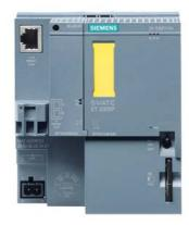
SIPLUS ET 200SP CPU 1510SP F-1PN based on 6ES7510-1SJ01-0AB0 with conformal coating, -25...+60 °C, central processing unit with work memory 150 KB for program and 750 KB for data, 1st interface, PROFINET IRT with 3-port switch, 72 ns bit performance, SIMATIC Memory Card required, BusAdapter required for port 1 and 2
