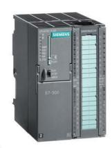
SIPLUS S7-300 CPU 313C-2DP based on 6ES7313-6CG04-0AB0 with conformal coating, -25...+70 °C, compact CPU with MPI, 16 DI/16 DQ, 3 high-speed counters (30 kHz), integrated DP interface, integrated power supply 24 V DC, work memory 128 KB, front connector (1x 40-pole) and Micro Memory Card required
