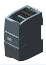
SIPLUS S7-1200 SM 1234 4AI/2AQ based on 6ES7234-4HE32-0XB0 with conformal coating, -20...+60 °C, analog I/O +/-10 V: 14-bit resolution or 0-20 mA: 13-bit resolution
