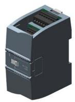
SIPLUS S7-1200 SM 1234 4AI/2AQ based on 6ES7234-4HE32-0XB0 with conformal coating, -40...+70 °C, start up -25 °C, analog I/O +/-10 V: 14-bit resolution 0-20 mA: 13-bit resolution
