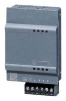
SIPLUS S7-1200 SB 1232 1AQ based on 6ES7232-4HA30-0XB0 with conformal coating, -40...+60 °C, start up -25 °C, analog output 1 AQ, +/-10 V DC (12 bit resolution) or 0-20 mA (11 bit resolution)
