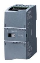
SIPLUS S7-1200 SM 1231 8AI based on 6ES7231-4HF32-0XB0 with conformal coating, -20...+60  $^{\circ}$ C, analog input SM 1231, 8 AI, +/-10 V, +/-5 V, +/-2.5 V, or 0-20 mA/4-20 mA, 12 bit+sign or (13 bit ADC)
