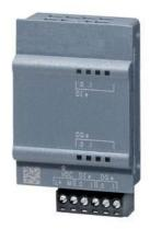
SIPLUS S7-1200 SB 1223 I/O based on 6ES7223-3AD30-0XB0 with conformal coating, -40...+60 °C, start up -25 °C, digital input/output 2 DI/2 DQ, 5 V DC 200 kHz
