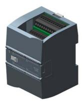
SIPLUS S7-1200 SM 1223 16DI/16DQ RLY based on 6ES7223-1PL32-0XB0 with conformal coating, -20...+60  $^\circ$ C, digital input/output 16 DI/16 DQ, 16 DI 24 V DC, sink/source, 16 DQ, relay 2 A
