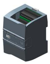
SIPLUS S7-1200 SM 1223 16DI/16DQ RLY based on 6ES7223-1PL32-0XB0 with conformal coating, -40...+70 °C, start up -25 °C, digital input/output 16 DI/16 DQ, 16 DI 24 V DC, sink/source, 16 DQ, relay 2 A
