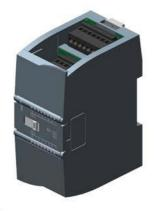
SIPLUS S7-1200 SM 1222 16DQ RLY based on 6ES7222-1HH32-0XB0 with conformal coating, -40...+70  $^{\circ}$ C, start up -25  $^{\circ}$ C, digital output 16 DQ, relay 2 A
