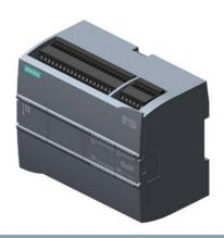
SIPLUS S7-1200 CPU 1215C DC/DC/relay based on 6ES7215-1HG40-0XB0 with conformal coating, -40...+60 °C, start up -25 °C, compact CPU, DC/DC/relay, 2 PROFINET ports, onboard I/O: 14 DI 24 V DC; 10 DQ relay 2 A; 2 AI 0-10 V DC, power supply: DC 20.4-28.8 V DC, program/data memory 125 KB
