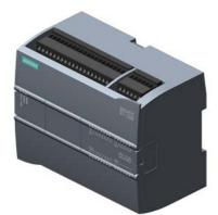
SIPLUS S7-1200 CPU 1215C AC/DC/relay based on 6ES7215-1BG40-0XB0 with conformal coating, -40...+60 °C, start up -25 °C, compact CPU, AC/DC/relay, 2 PROFINET ports onboard I/O: 14 DI 24 V DC; 10 DQ relay 2 A; 2 AI 0-10 V DC, 2 AQ 0-20 mA DC power supply: AC 85-264 V AC @ 47-63 Hz, program/data memory 125 KB
