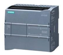
SIPLUS S7-1200 CPU 1214C DC/DC/relay based on 6ES7214-1HG40-0XB0 with conformal coating, -40...+60 °C, start up -25 °C, compact CPU, DC/DC/relay, onboard I/O: 14 DI 24 V DC; 10 DQ relay 2 A; 2 AI 0-10 V DC, power supply: AC 20.4-28.8 V DC, program/data memory 100 KB
