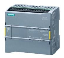
SIPLUS S7-1200 CPU 1214FC DC/DC/relay based on 6ES7214-1HF40-0XB0 with conformal coating, -25...+55 °C, compact CPU, DC/DC/relay, onboard I/O: 14 DI 24 V DC; 10 DQ relay 2 A; 2 AI 0-10 V DC, power supply: DC 20.4-28.8 V DC, program/data memory 125 KB
