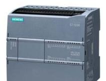
SIPLUS S7-1200 CPU 1214C AC/DC/relay based on 6ES7214-1BG40-0XB0 with conformal coating, -40...+70 °C, start up -25 °C, signal board: 0, compact CPU, AC/DC/relay, onboard I/O: 14 DI 24 V DC 10 DQ relay 2 A 2 AI 0-10 V DC, power supply: AC 85-264 V AC @ 47-63 Hz, program/data memory 100 KB
