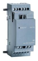
SIPLUS LOGO! AM2 AQ based on 6ED1055-1MM00-0BA2 with conformal coating, -40...+70 °C, start up -25 °C, expansion module, PS: 24 V DC, 2 AQ, 0-10 V, 0/4-20 mA for LOGO! 8
