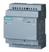
SIPLUS LOGO! 230RCEO based on 6ED1052-2FB08-0BA1 with conformal coating, -40...+70 °C, start up -25 °C, logic module, power supply / I/O: 115V/230V/relay, 8 DI/4 DQ, without display, memory 400 blocks, modularly expandable, Ethernet, integrated web server, data log, user-defined web pages, standard microSD card for LOGO! Soft Comfort V8.3 or higher older projects executable cloud connection in all LOGO! 8.3 basic unit
