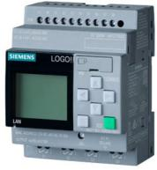
SIPLUS LOGO! 12/24RCE based on 6ED1052-1MD08-0BA1 with conformal coating, -25...+60 °C, start up -20 °C, logic module, display power supply / I/O: 12/24 V DC/relay, 8 DI (4 Al)/4 DQ, memory 400 blocks, modularly expandable, Ethernet, integrated web server, data log, user-defined web pages, standard microSD card for LOGO! Soft Comfort V8.3 or higher, older projects executable cloud connection in all LOGO! 8.3 basic units
