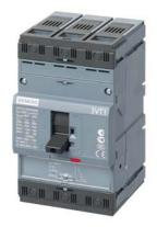
circuit breaker 3VT1 standard breaking capacity Icu=25kA, 415V AC 3-pole, line protection trip unit TM, LI In=80A rated current IR=63...80A overload protection II=400...800A, short-circuit protection without auxiliary release without auxiliary/alarm switch
