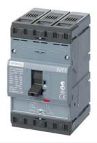
circuit breaker 3VT1 standard breaking capacity Icu=25kA, 415V AC 3-pole, line protection trip unit TM, LI In=63A rated current IR=50...63A overload protection II=315...630A, short-circuit protection without auxiliary release without auxiliary/alarm switch
