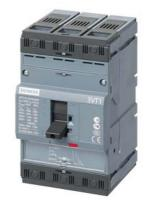
circuit breaker 3VT1 standard breaking capacity Icu=25kA, 415V AC 3-pole, line protection trip unit TM, LI In=63A rated current IR=50...63A overload protection II=315...630A, short-circuit protection without auxiliary release without auxiliary/alarm switch
