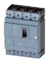
circuit breaker 3VM1 IEC frame 630 breaking capacity class N Icu=36kA @ 415V 4-pole, line protection TM220, ATFM, In=500A overload protection Ir=350A...500A short-circuit protection Ii=10 x In N conductor protection 100% nut keeper kit
