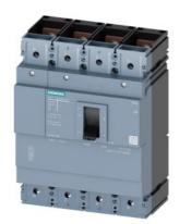
circuit breaker 3VM1 IEC frame 630 breaking capacity class N Icu=36kA @ 415V 4-pole, line protection TM210, FTFM, In=500A overload protection short-circuit protection li=10 x In N conductor protection 100% nut keeper kit
