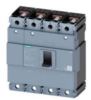
circuit breaker 3VM1 IEC frame 250 breaking capacity class M Icu=55kA @ 415V 4-pole, line protection TM210, FTFM, In=250A overload protection Ir=250A, not adjustable short-circuit protection li=10 x In N conductor protection 100% nut keeper kit
