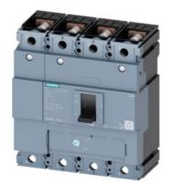
circuit breaker 3VM1 IEC frame 250 breaking capacity class S Icu=36kA @ 415V 4-pole, line protection TM220, ATFM, In=250A overload protection Ir=175A...250A short-circuit protection Ii=10 x In N conductor protection 100% nut keeper kit
