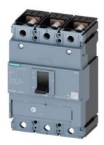
circuit breaker 3VM1 IEC frame 250 breaking capacity class S Icu=36kA @ 415V 3-pole, line protection TM220, ATFM, In=250A overload protection Ir=175A...250A short-circuit protection Ii=10 x In nut keeper kit
