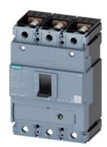
circuit breaker 3VM1 IEC frame 250 breaking capacity class M Icu=55kA @ 415V 3-pole, starter protection TM120M, AM, In=200A without overload protection short-circuit protection Ii=6...14 x In nut keeper kit
