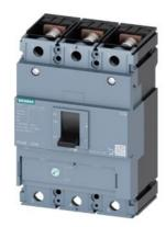
circuit breaker 3VM1 IEC frame 250 breaking capacity class M Icu=55kA @ 415V 3-pole, line protection TM220, ATFM, In=200A overload protection Ir=140A...200A short-circuit protection Ii=10 x In nut keeper kit
