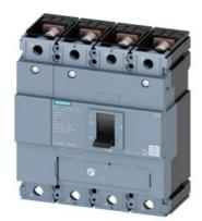
circuit breaker 3VM1 IEC frame 250 breaking capacity class S Icu=36kA @ 415V 4-pole, line protection TM220, ATFM, In=200A overload protection Ir=140A...200A short-circuit protection Ii=10 x In N conductor protection 100% nut keeper kit
