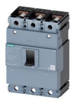
circuit breaker 3VM1 IEC frame 250 breaking capacity class S Icu=36kA @ 415V 3-pole, line protection TM210, FTFM, In=200A overload protection Ir=200A, not adjustable short-circuit protection Ii=10 x In nut keeper kit
