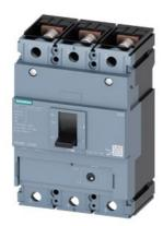
circuit breaker 3VM1 IEC frame 250 breaking capacity class M Icu=55kA @ 415V 3-pole, starter protection TM120M, AM, In=160A without overload protection short-circuit protection Ii=7...16 x In nut keeper kit
